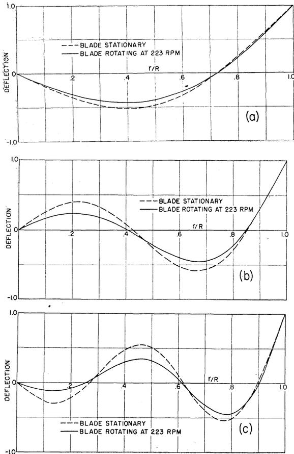
FIG. 9. Beamwise natural modes. (a) Fundamental mode, (b) second mode, (c) third mode.
