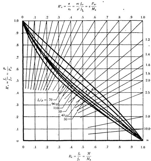
Reduced Interaction Curves for Combined Bending and Axial Loading
