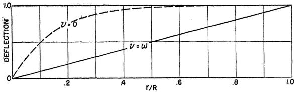
FIG. 8. Rigid blade mode and static mode of rotating blade at  $\omega = 223$  r.p.m., beamwise.
