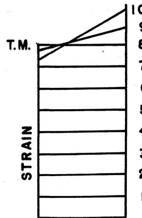
FIG. 7. Type of strain distribution needed to permit loading beyond tangent-modulus load.
