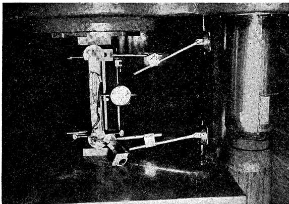
FIG. 3. Pin-end column test arrangement.
