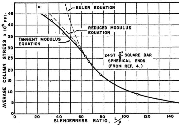
FIG. 2. Column theories and test data (Van den Broek).
