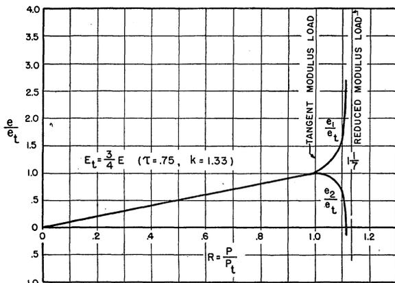
FIG. 11. Calculated strain variation with column load for a hypothetical column.
