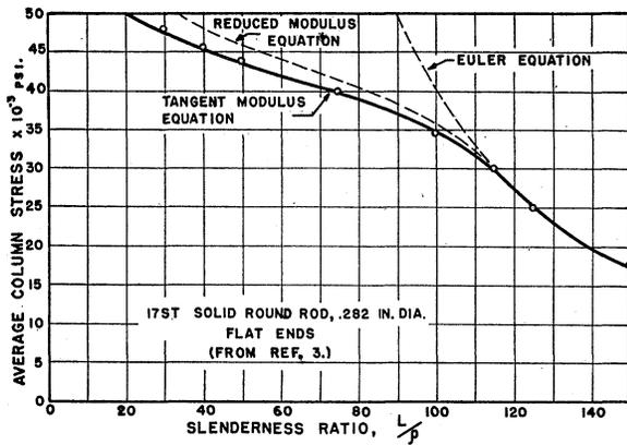
FIG. 1. Column theories and test data (Alcoa).
