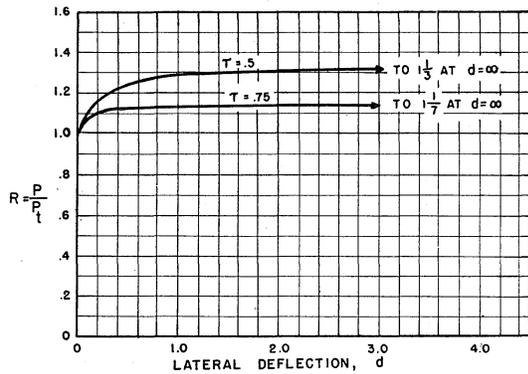
FIG. 10. Variation of column load with lateral deflection, assuming  $E_t$  constant.
