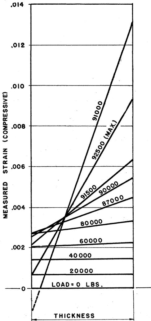
FIG. 4. Strain distribution as determined in a column test.
