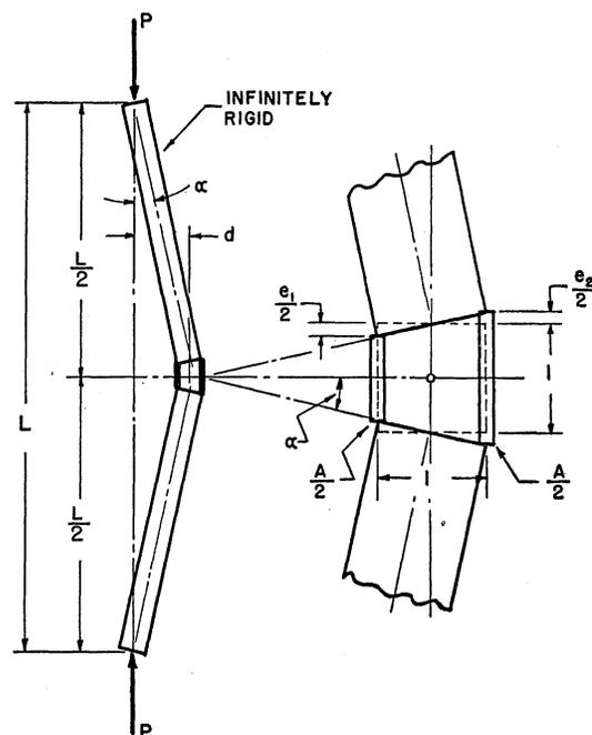
FIG. 9. Simplified two-flange column.
