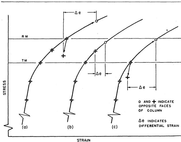
FIG. 8. Alternative types of strain progression.
